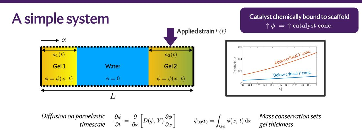
Applying a strain changes the interfacial boundary condition and so deswells gel 2
